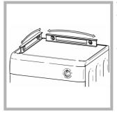
When you have installed your dryer in its final location check that it is level first side to side, then front to back.
